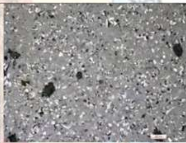
Fig.4.2 Tiny magnetites disseminated in the basaltic matrix
